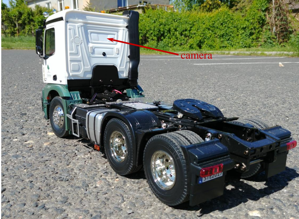
Figure 5. View of the camera for recognizing the semi-trailer
